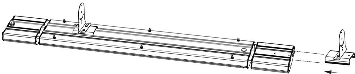
Step 3: Fix adjusting bracket into the wall by expansion screws.
