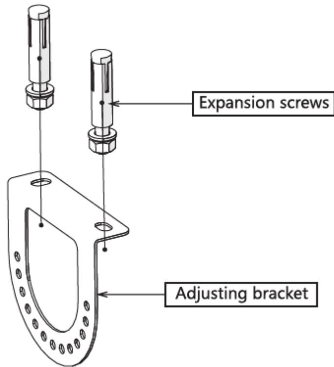
Step 4: Installation of two adjusting brackets; make sure lock brackets tight by butterfly hand screw.
