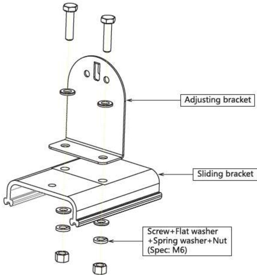
Step 2: Installation of sliding bracket & heater, as arrow points.
